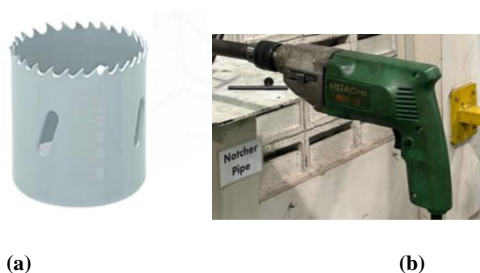
Figure 2: Bi-metal hole saw cutting tool (a) and Hitachi DUT-13 hand drill as the notching machine drive unit (b)
