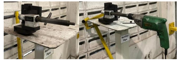
Figure 3: Pipe notching machine (a) and manual pipe notching machine setup (b)
