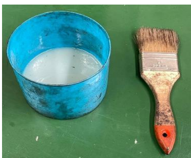
Figure 12: Cutting fluid applied manually using a brush
