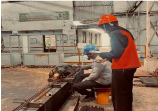
Figure 2: Noise measurement process using sound level meter
