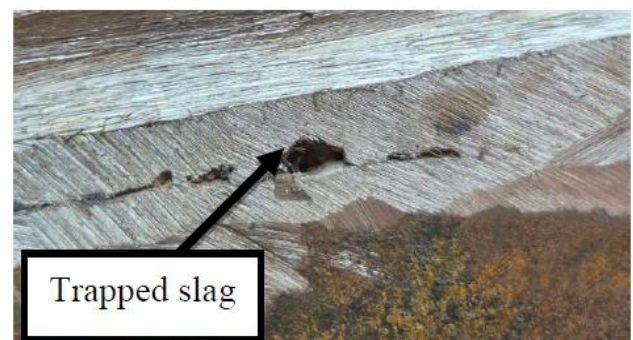
Figure 5: Slag Inclusion welding defect
